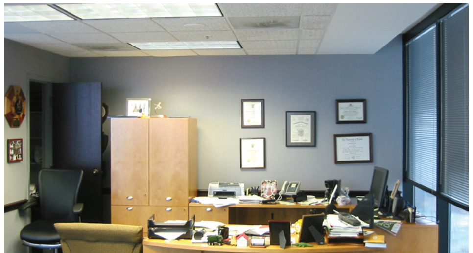
Ceiling lights with parabolic louvers reduce glare but often light the wrong surfaces.
